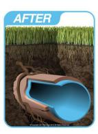
The cleaned pipes are lined with resin saturated liner. The liner cures via steam. Robotic equipment is used to reopen branch lines.
